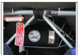
The system is activated by pulling the red handle. It is located either overhead the pilots seats (see picture) or at the center console. The safety pin must be removed before flight. The safety pin should be installed again during storage / parking of the aircraft to avoid inadvertent activation.
