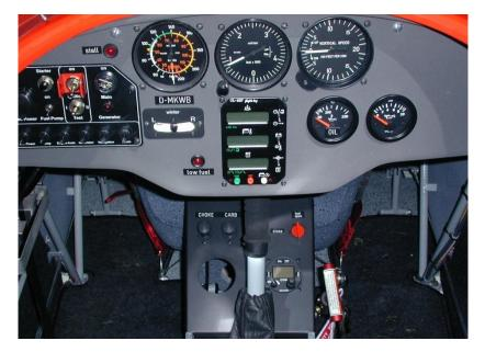
Controls to operate flaps, throttle and trim are located at the sidewall.
