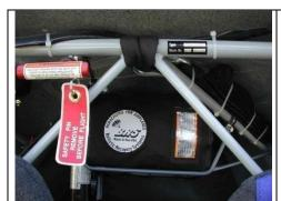
The system is activated by pulling the red handle overhead the pilots seats. The safety pin must be removed before flight. The safety pin should be installed again during storage / parking of the aircraft to avoid inadvertent activation.
