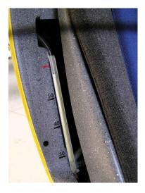
planning purposes. This gauge indicates less than full with tanks completely filled.
