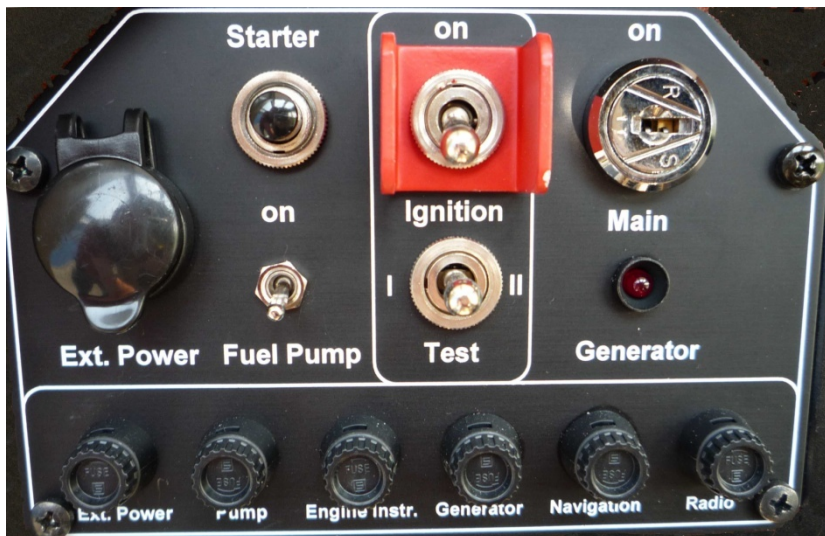
Ext. Power Pump Eng.Instr. Generator Navigation Radio 2A 8A 500mA 500mA 2A 2A
